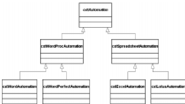
Figure 2. In this class hierarchy, the cstAutomation class provides the interface that’s common to all types of Automation servers. Beneath that are abstract class definitions with interfaces for different types of applications, with the implementation-level classes being specific to a certain vendor’s applications.
