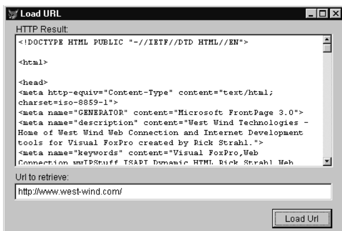
Figure 7.1. Using WinInet to pull a Web page to a string takes only two lines of code using the wwIPStuff class.
