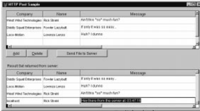
Figure 7.4. Sending and receiving data files over HTTP is easy. This form allows entering of data to send to the server, which adds a record and then returns the full result for display in the lower grid.
