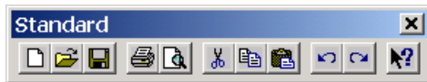
Figure 2. Invisible separators—the Style property for the separators in this toolbar is set to 0-Normal .
