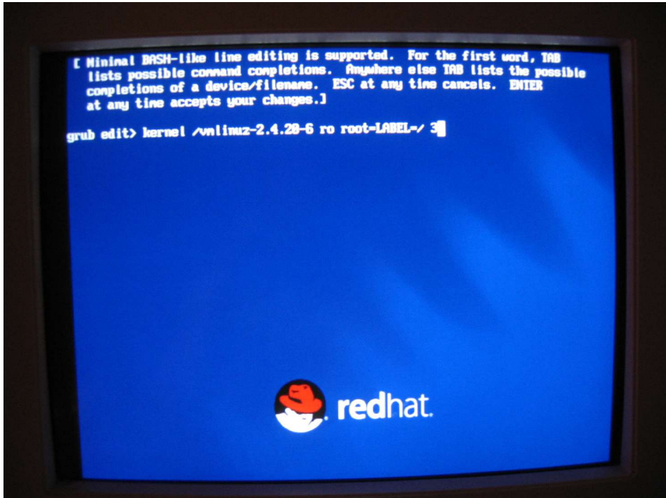
Figure 10. Enter the number of the runlevel you want to boot into, after typing a space.
