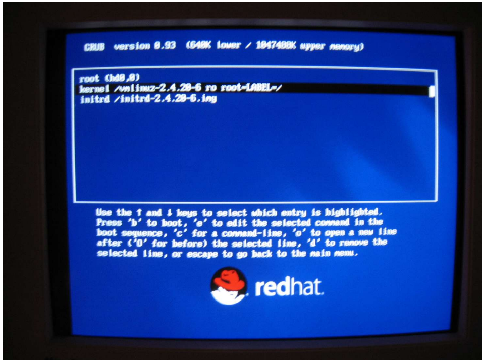
Figure 8. Move the highlight to the line beginning with 'kernel' in order to change the runlevel.
