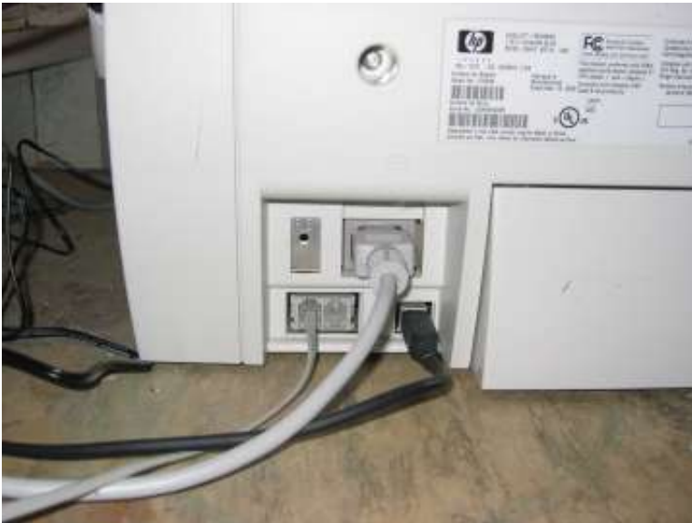
Figure 5. The back of the Hewlett-Packard LaserJet 3200 shows the connection of the USB cable.
