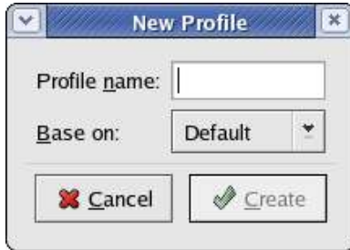
Figure 1. The New Profile dialog allows you to create a new profile, and optionally base it on an existing profile.
