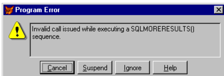
Figure 7. The results of trying to issue another SQL pass through function while processing result sets in non-batch mode.
