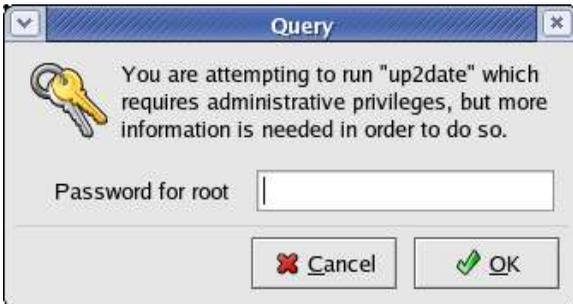
Figure 19. First, log in as root in order to run up2date.
