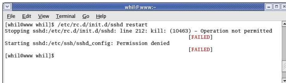
Figure 6. You can't restart SSH on the remote machine unless you're logged in as root.
