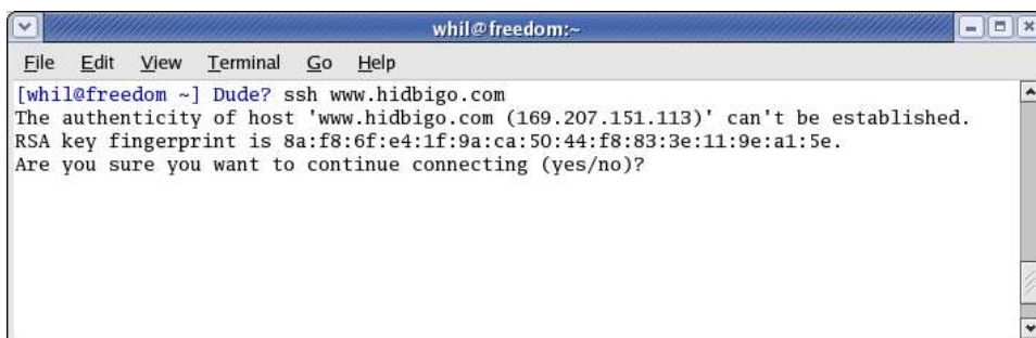
Figure 2. Upon first connection, you're asked to confirm this is the machine you want to connect to.
