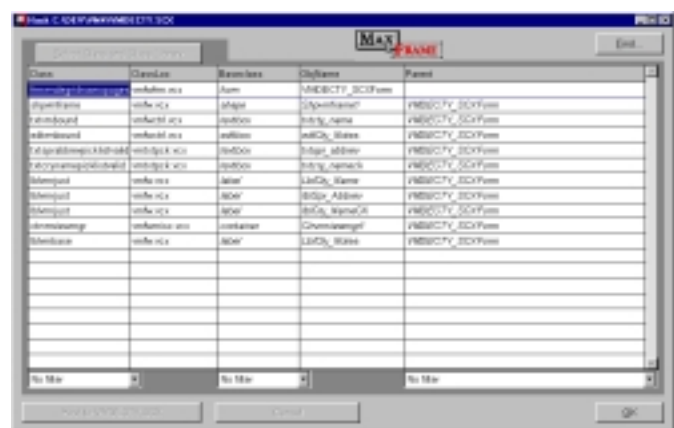
Figure 6. Developers can use the “hacking” tool to change the parent class of contained objects.
